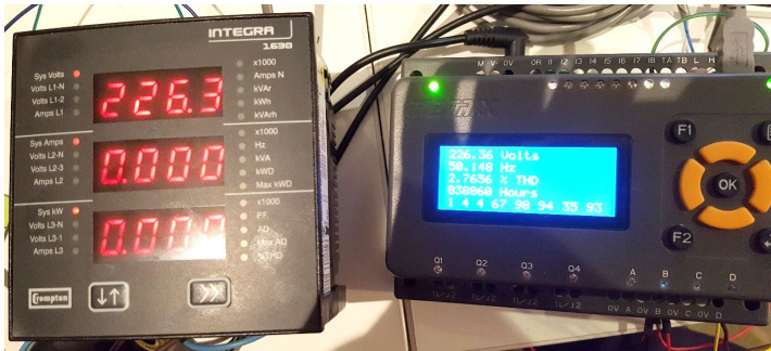
A 16-bit dsPIC® DSC MIAC automates key tasks for an independent source of mains power in Australia.
