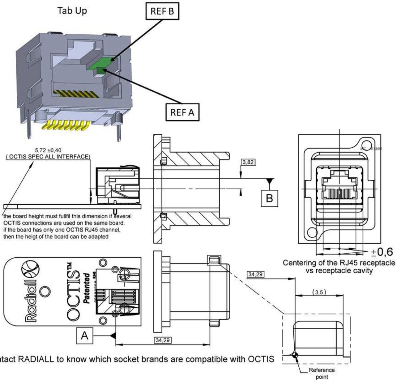
Contact RADIALL to know which socket brands are compatible with OCTIS
