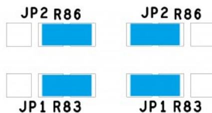
Figure 14a. DAC clock is connected to on-board oscillator (default) | Figure 14b. DAC clock is connected to J10
