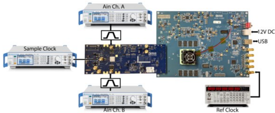
Figure 2. ADS8-V1 connected to High Speed A/D Converter Evaluation Board
