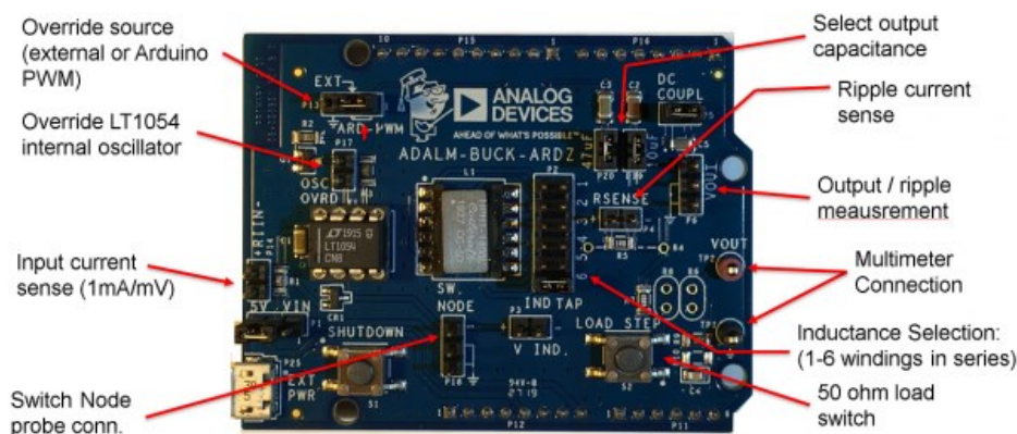
Figure 1. ADALM-BUCK connections and jumpers
