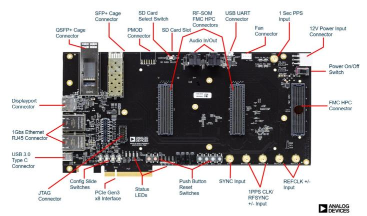
The ADRV2CRR-FMC is the carrier board to allow users evaluate the functionality of the ADRV9009-ZU11EG RF-SOM. It contains common high speed I/O ports to give flexibility in what connectivity option the user needs. It comes with a power supply that powers up the full system, heatsink that the user fits to the RFSOM heat spreader plate and necessary cables and adapters to get up and running.
