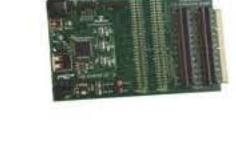
The Microchip PIC32 Accessory Development Start Kit for Android™ is used for evaluating and developing accessories for Google's Android operating system for smartphones and tablets.
