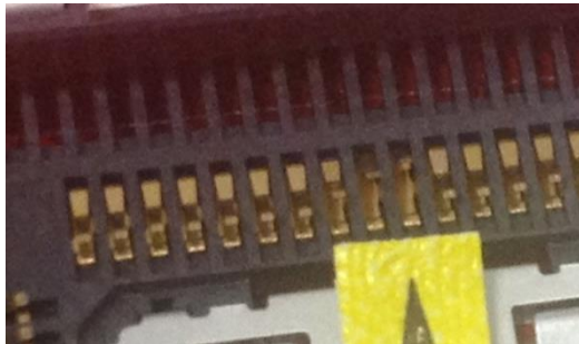
Figure 16. Example of Bent Contacts
