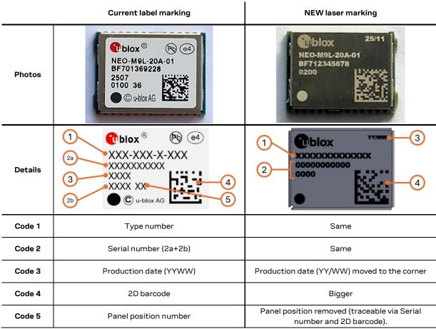
Table 1: comparison between current label-marking and new laser-marking.
